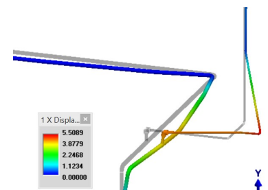
Displacement due to Relief Valve Firing
