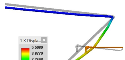
Displacement due to Relief Valve Firing
