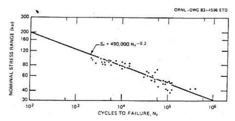
Equation 1 has been normalized based on the peak stress range in a girth butt-weld (i.e. i = 1.0). As a result, there is an inherent factor on the peak stress range "S" of 0.50. All peak stresses given by Markl SIFs are half of their actual values due to Markl's use of girth butt-welds as a baseline.
